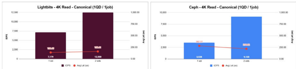
Figure 2: Canonical 4K Random Read (QD=1) IOPS and average latency for Lightbits and Ceph.
